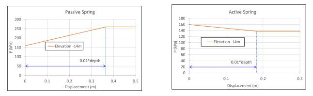
Figure 5: Lateral Earth Pressure – Displacement Variations for Liquefied Soil
