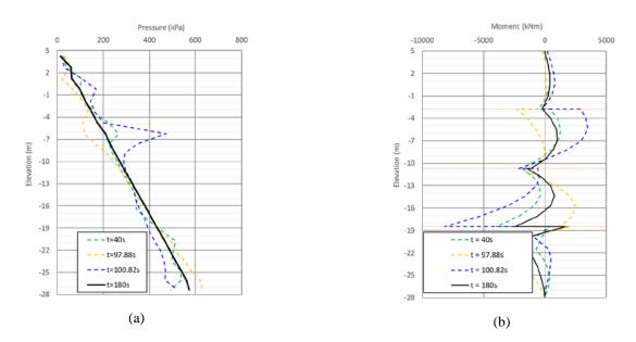
Figure 2: (a) Earth pressures and (b) bending moment profiles on the dumper wall at different time step during shaking
